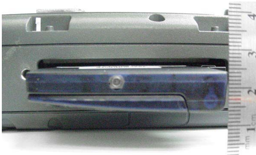
AirCard 580 Card-to-Base Distance (Broadband Hatch & Antenna Removed)
