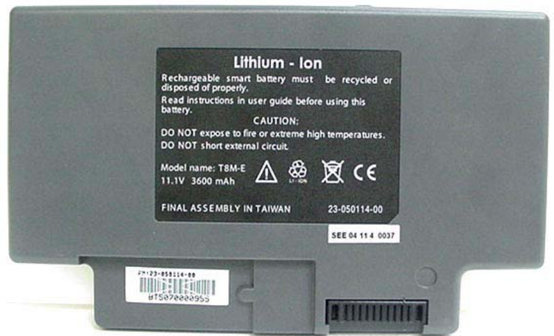
Internal Lithium-ion Battery (Model: T8M-E)
