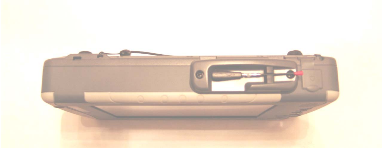
'Top View IX300 AC775 Antenna visible
