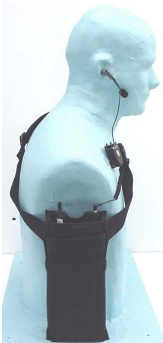
Front Side of DUT facing body - worst-case antenna configuration relative to right arm
