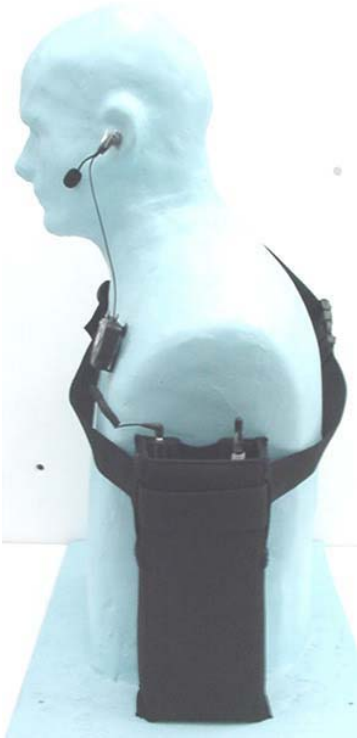
Back Side of DUT facing body - worst-case antenna configuration relative to left arm
