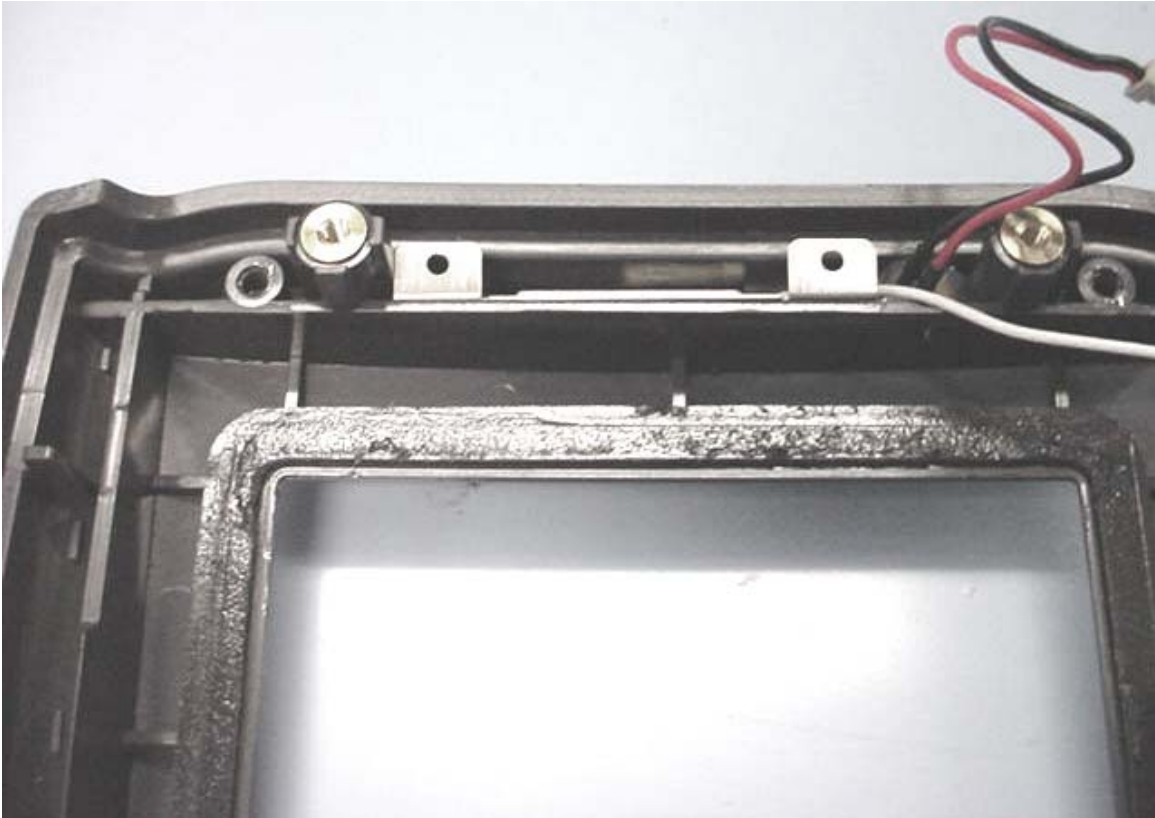
802.11b Internal Antenna Location
