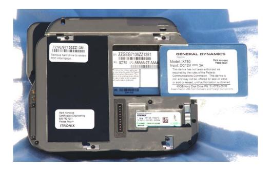
Battery on the left below, bottom of the IX750 on the right hard drive removed
