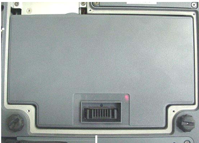
Internal Li-ion Battery 11.1 V, 3600 mAh (Model: T8M-E)
