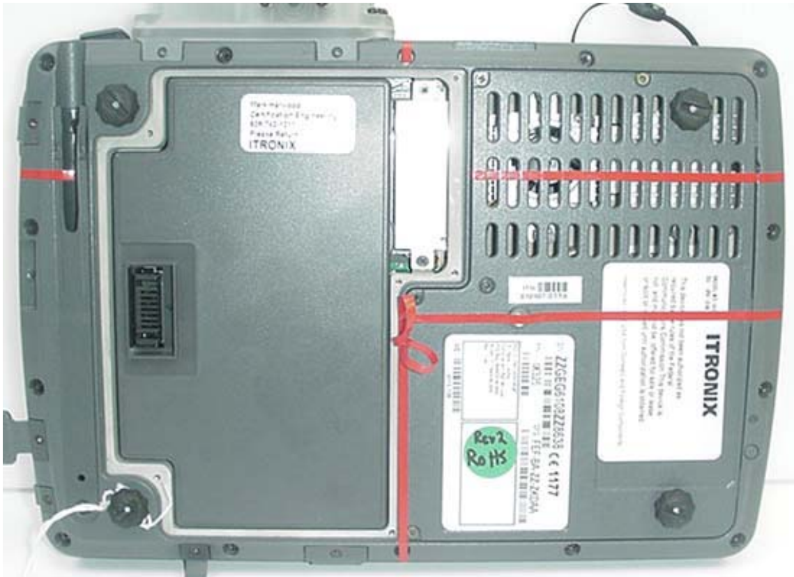
Bottom Side of DUT with Internal Li-ion Battery 11.1 V, 3600 mAh (Model: T8M-E)
