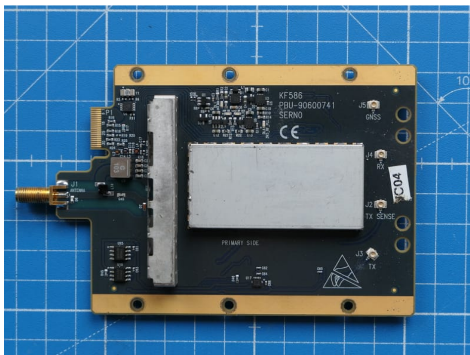
Photo 16: PCB 5 with shielding
