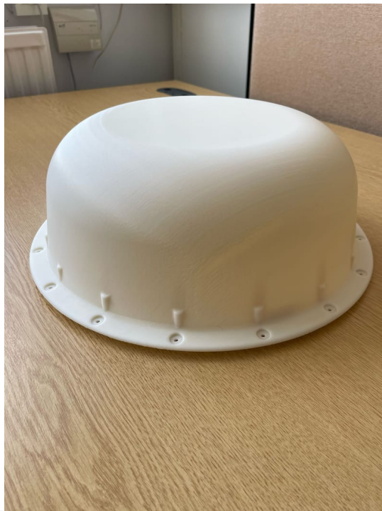
Photo 14: SpaceCom Class 7 Antenna Radome
