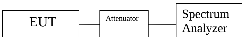
Figure 4. Block Diagram, Occupied Bandwidth Test Setup
