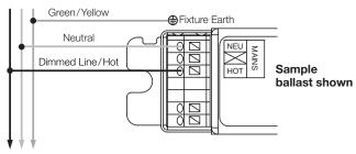
NOTE: Output must NOT be used to control receptacles. Output must be directly connected to the load. Output breakers or switches must not be used.
