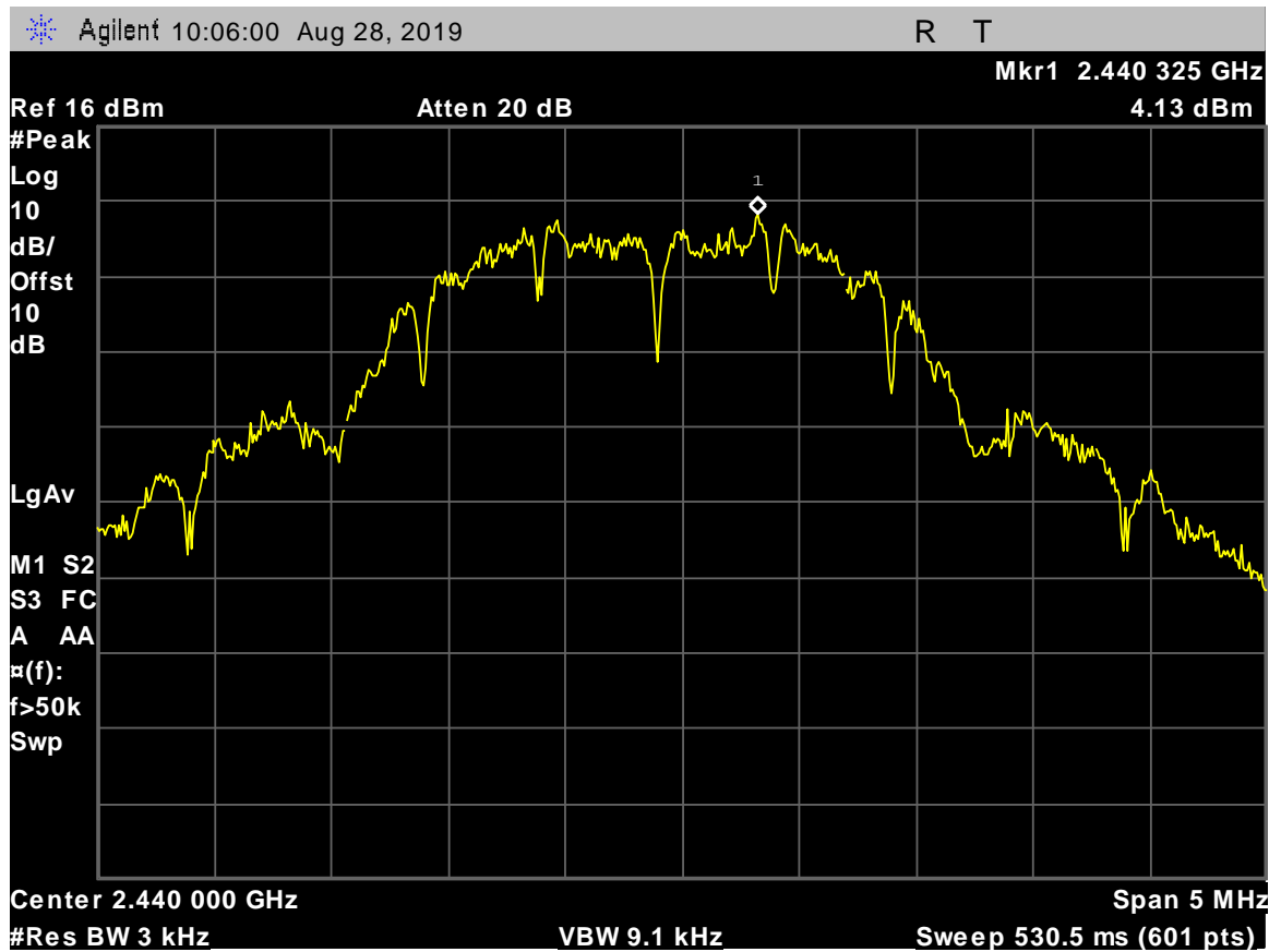
Figure 48: Peak Power Spectral Density, ANT2, 2440 MHz
