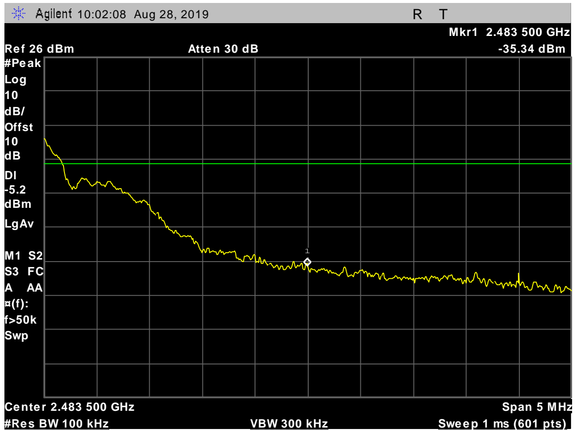
Figure 45: Spurious Emissions in Non-restricted Bands, 100 KHz, ANT2, 2480 MHz, High Band Edge
