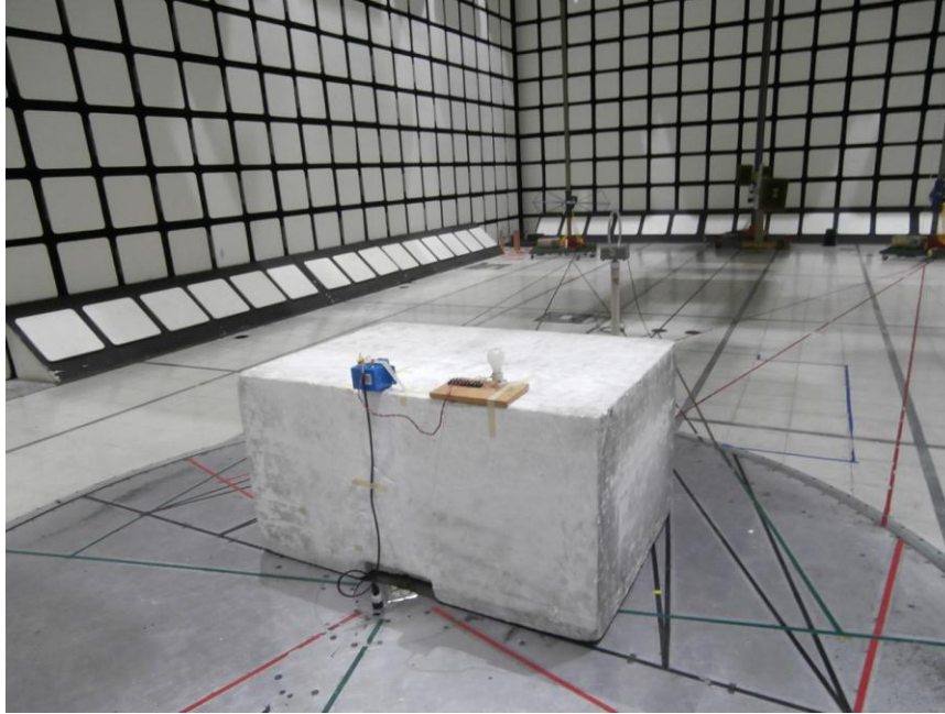
RADIATED EMISSIONS BELOW 30MHz (BACK)
