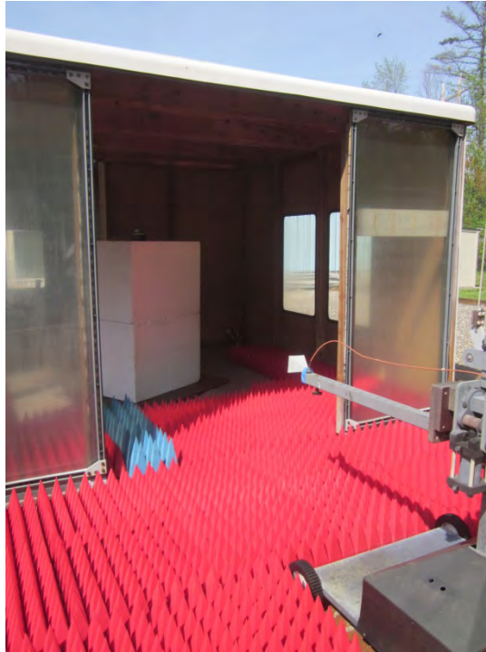
Horizontal Antenna Polarization, 18 GHz to 25 GHz, Horn
