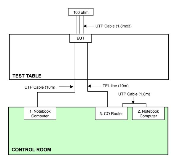
**NOTE:** 1. Support units 1-3 were kept in the control room during the test.
