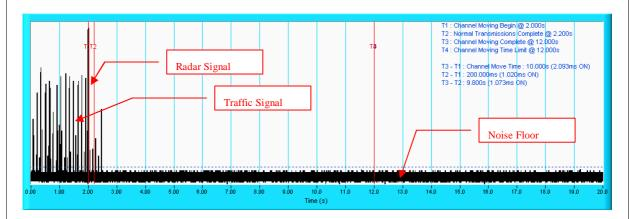
**NOTE:** T1 denotes the start of Channel Move Time upon the end of the last Radar burst. T2 denotes the data transmission time of 200ms from T1. T4 denotes the 10 second from T1 to observe the aggregate duration of transmissions.
