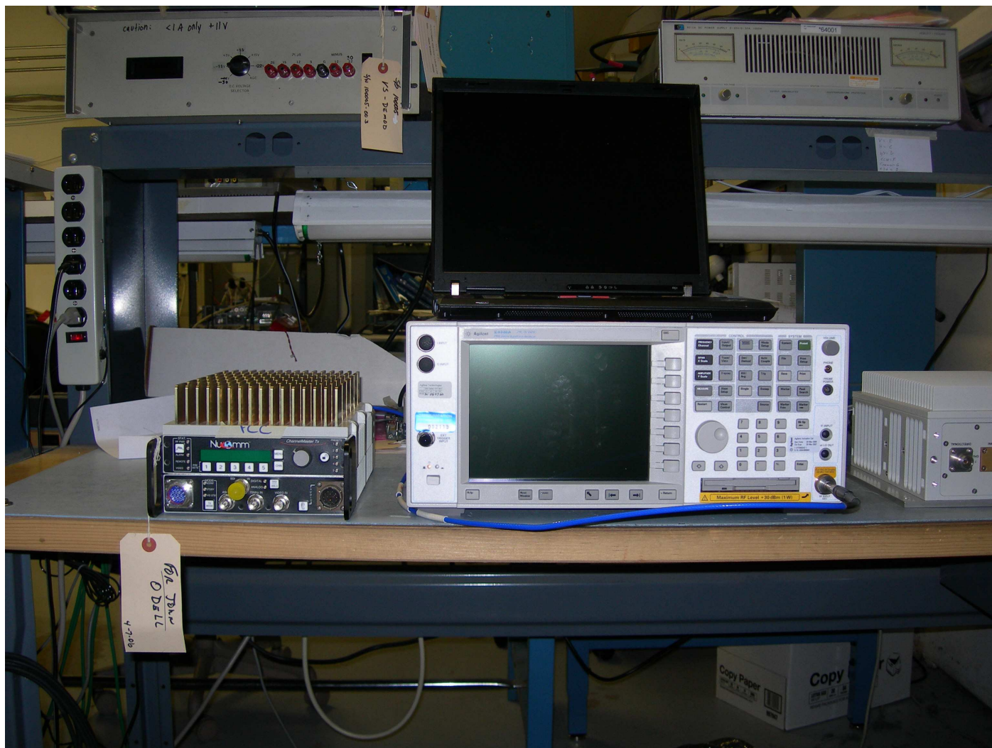
Figure 1: Test setup for Occupied Bandwidth, Conducted Emissions, and Output Power Levels
