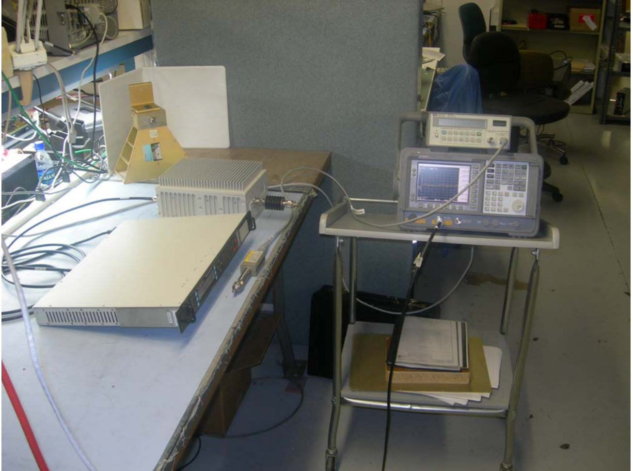
Test setup for Occupied Bandwidth, Conducted Emissions, and Output Power Levels
