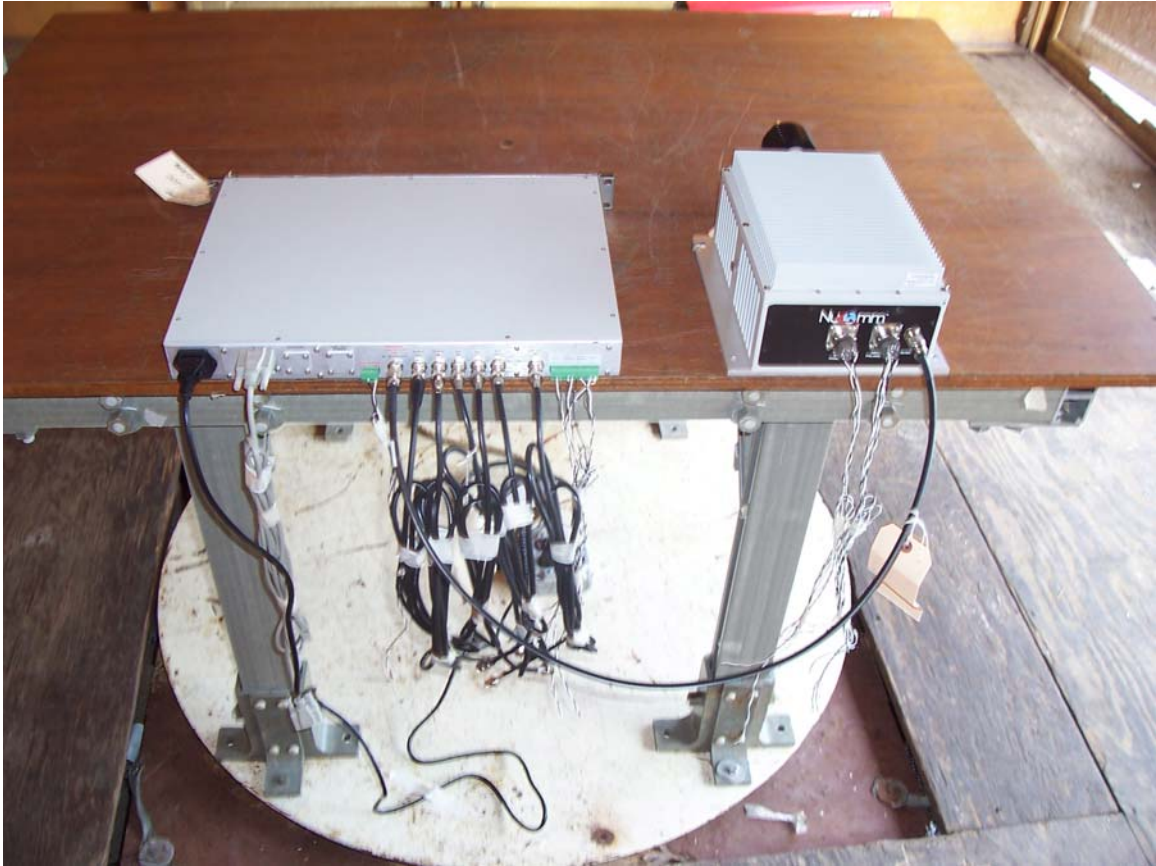
Test setup used for Spurious Emissions (back)
