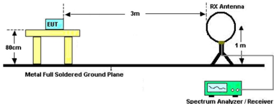
For radiated emissions from 30MHz to 1GHz
