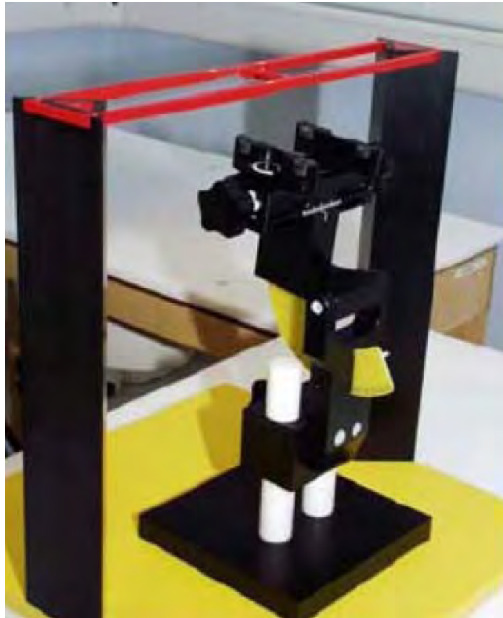
Figure 7 T-coil Phantom & Device Holder
