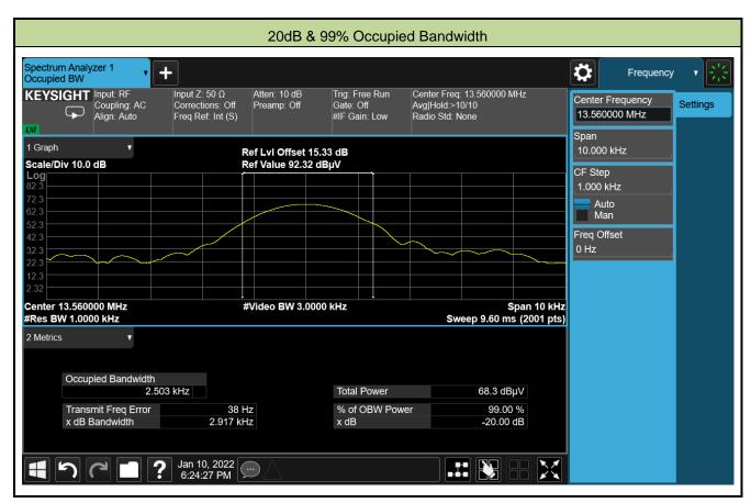
Note: Because the measured signal is CW adjusting the RBW per C63.10-2013 would not be practical since measured bandwidth will always follow the RBW and the result will be approximately twice the RBW.
