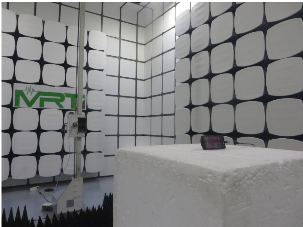
Description: Radiated Spurious Emissions Test Setup (above 1GHz)
