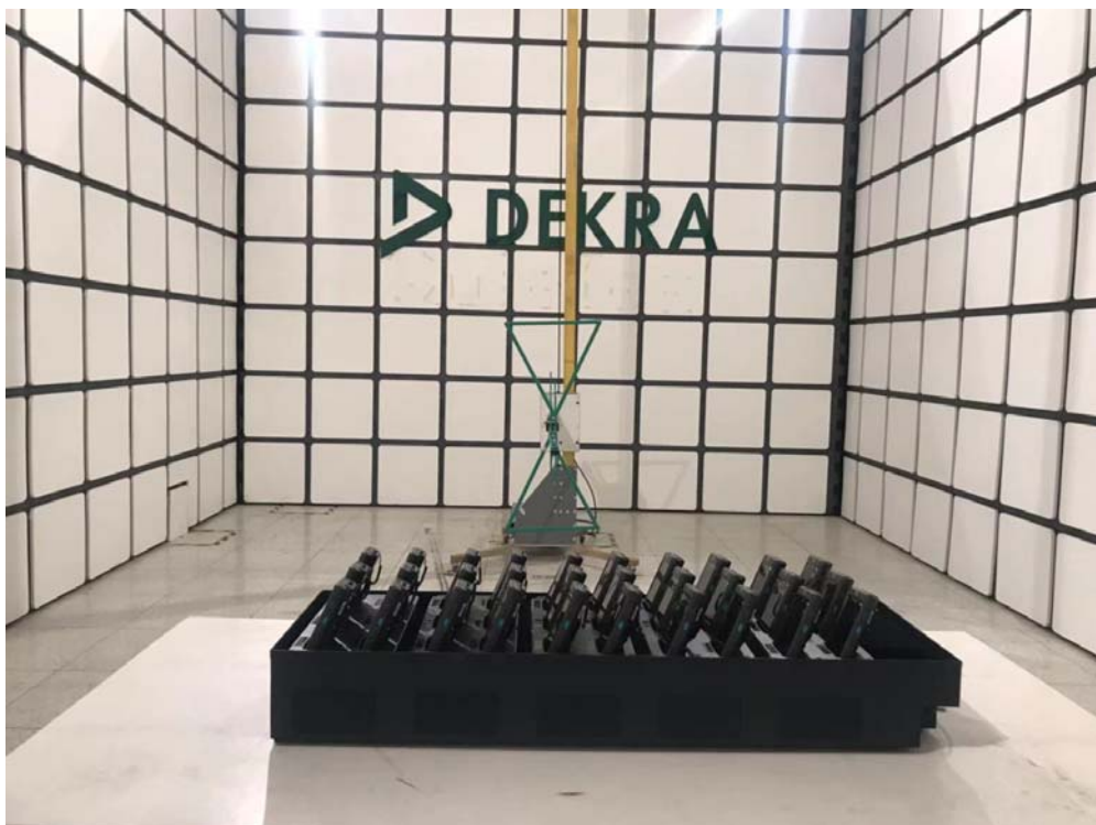
Description: Radiated Emission Test Setup for Above 30MHz
