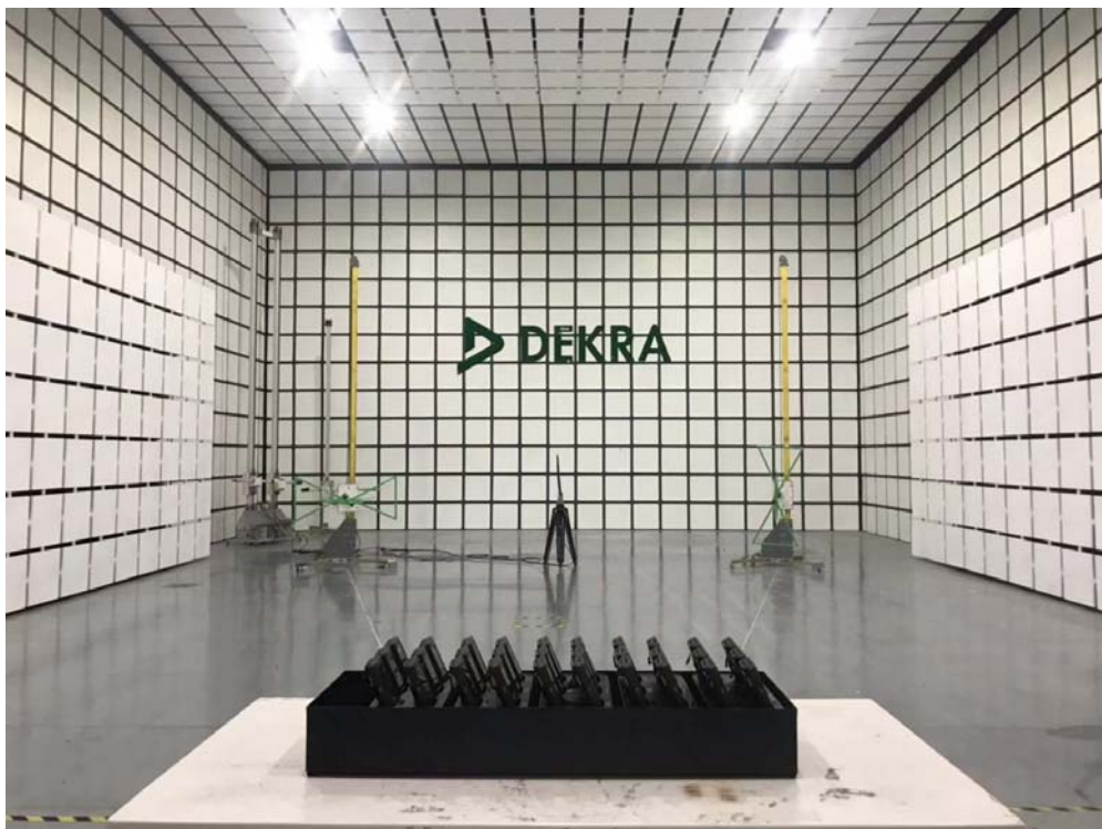
Description: Radiated Emission Test Setup for Above 30MHz
