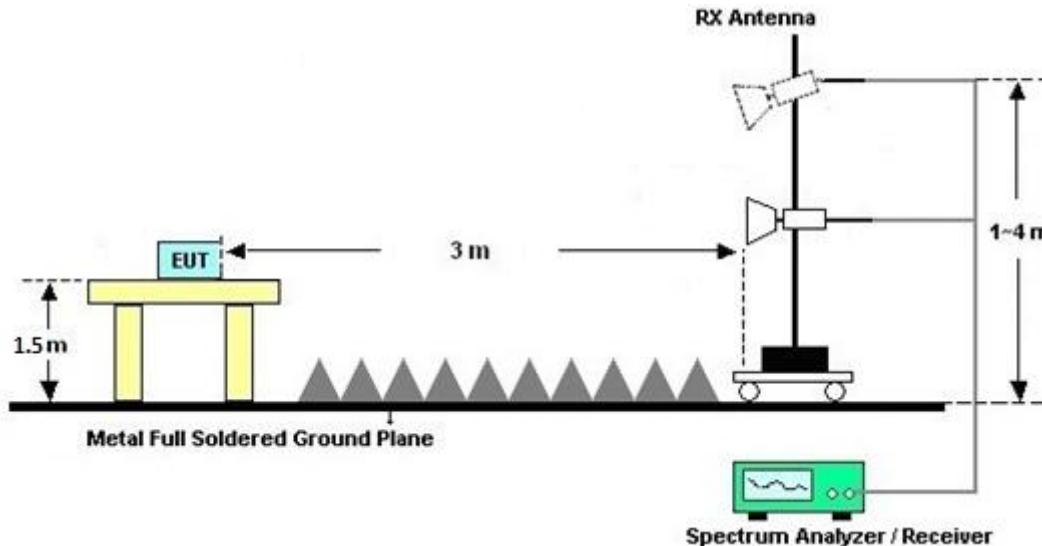
For radiated test above 18GHz
