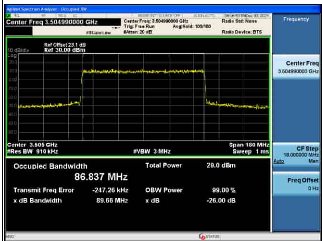
OCC_5G_n77(K)_30KHz_64QAM_10M CH630334
