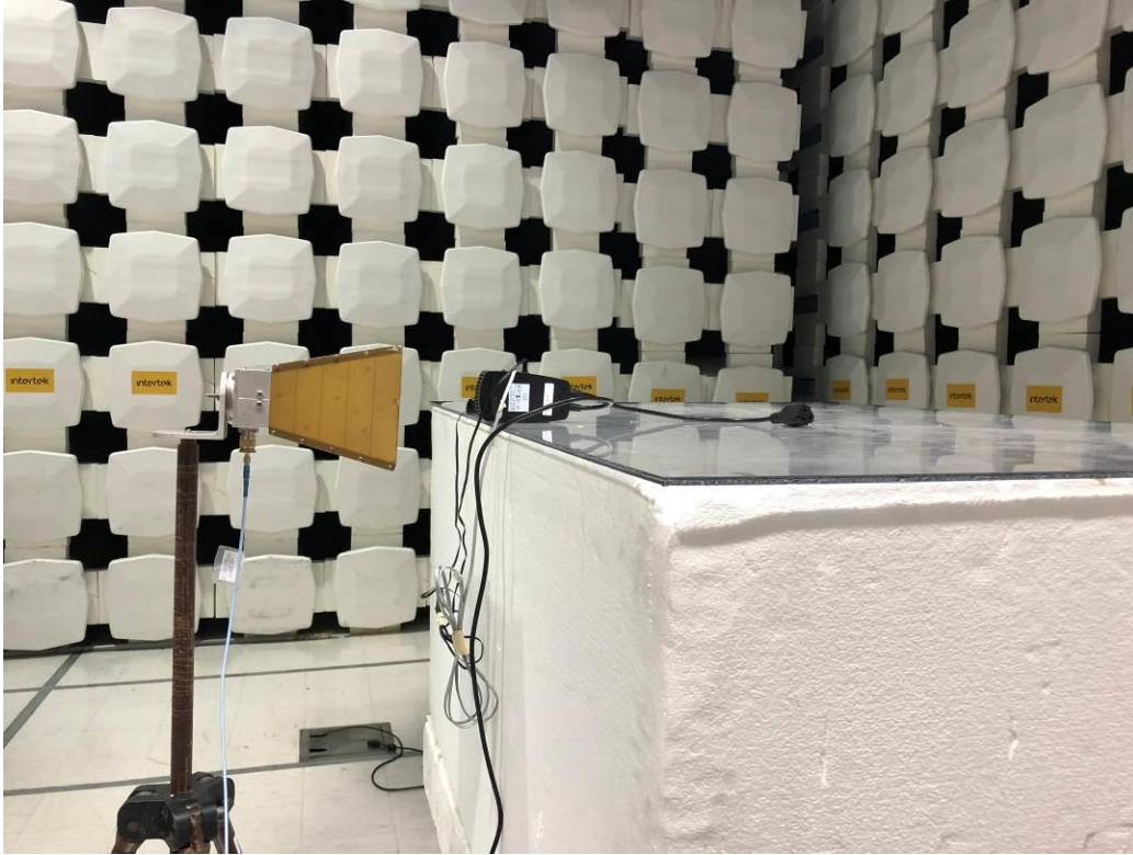
Radiated Emissions Worst-case Test Setup (Manual Testing), 9-18 GHz
