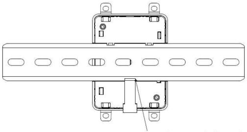
Move active clip to upward to fasten Dali module on din rail
