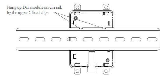
3. Move active clip to upward to fasten Dali module on din rail.
