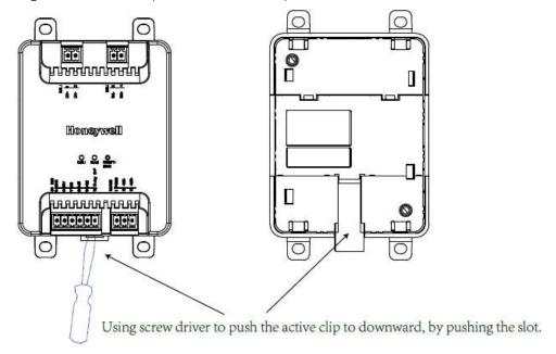
2. Hang up Dali module on din rail, by the upper 2 fixed clips.
