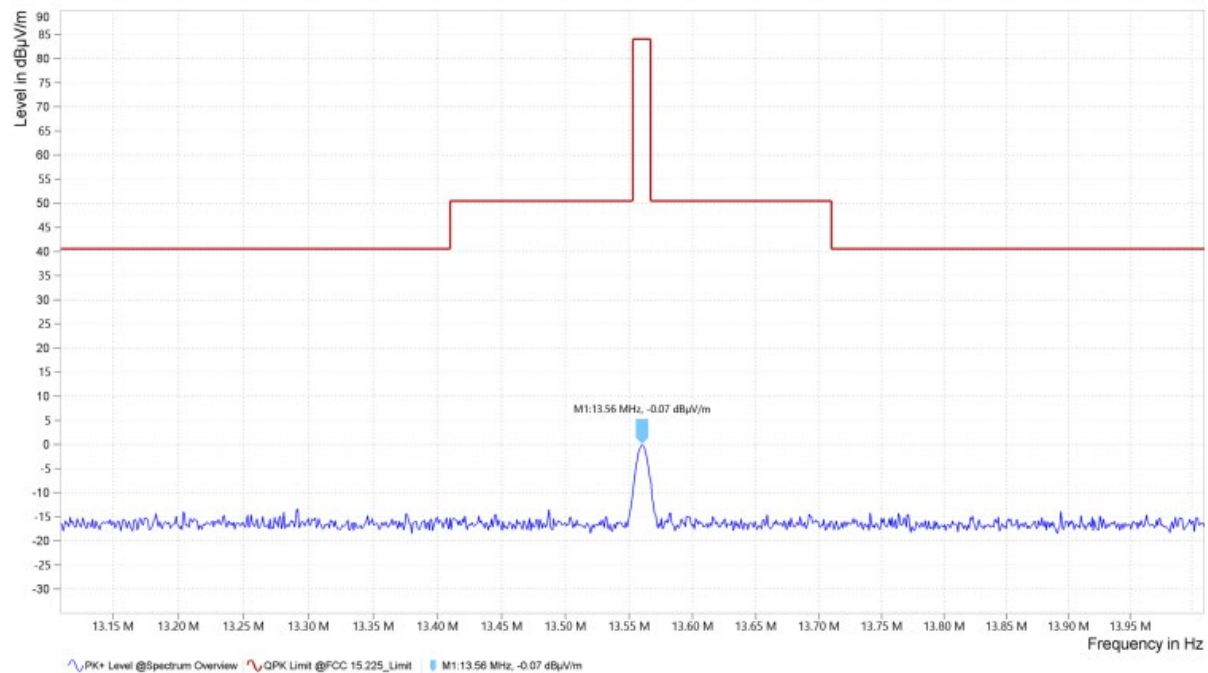
Figure 9-5 Carrier Mask without Load CW mode (13.56 MHz)-Antenna Parallel Orientation
