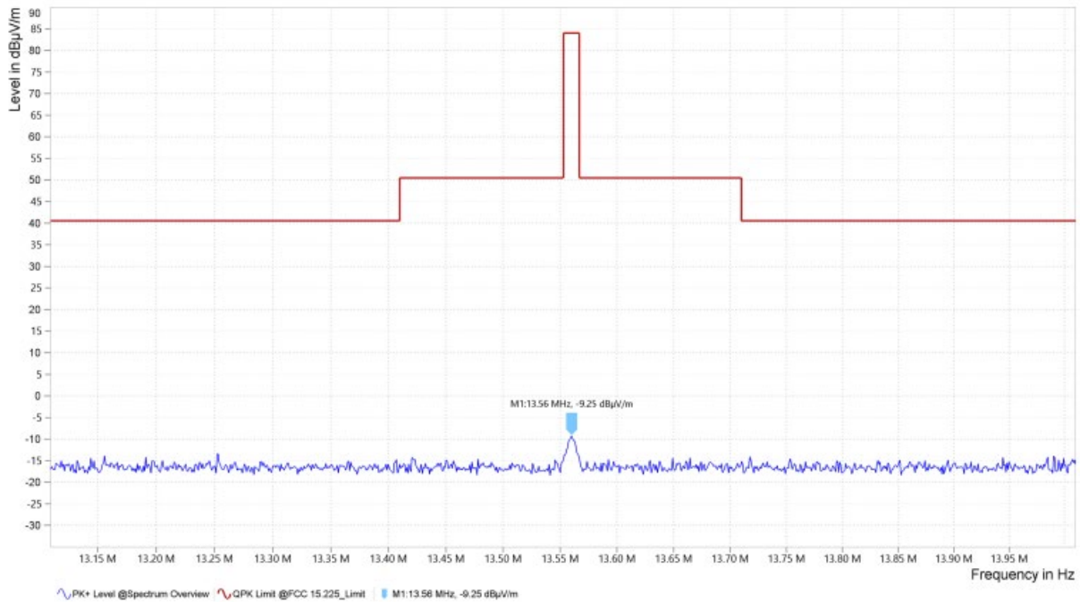
Figure 9-4 Carrier Mask with Load ASK modulation (13.56 MHz)-Antenna Parallel Orientation
