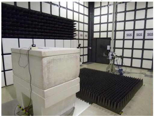
Radiated Emission Set up Photos (Front View)
