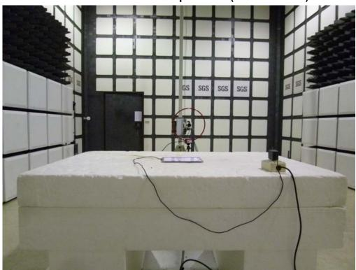
Radiated Emission Set up Photos (Below 1GHz)
