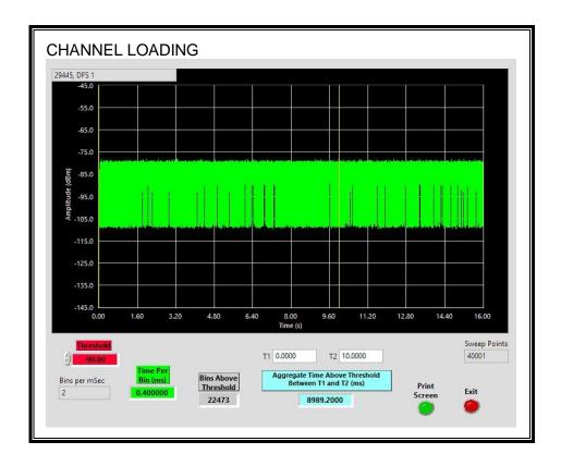
The level of traffic loading on the channel by the EUT is 88.89%
