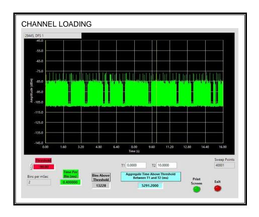
The level of traffic loading on the channel by the EUT is 52.91%
