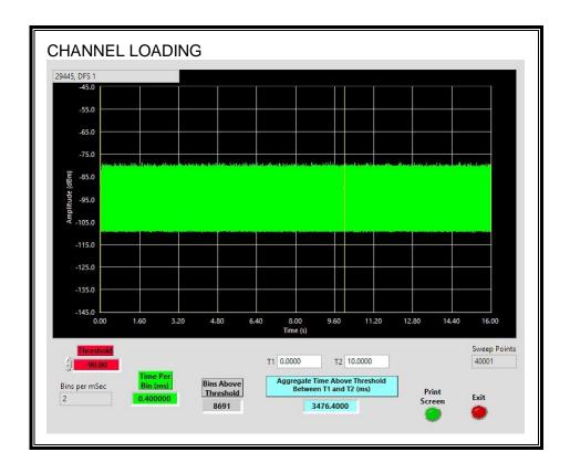
The level of traffic loading on the channel by the EUT is 34.76%
