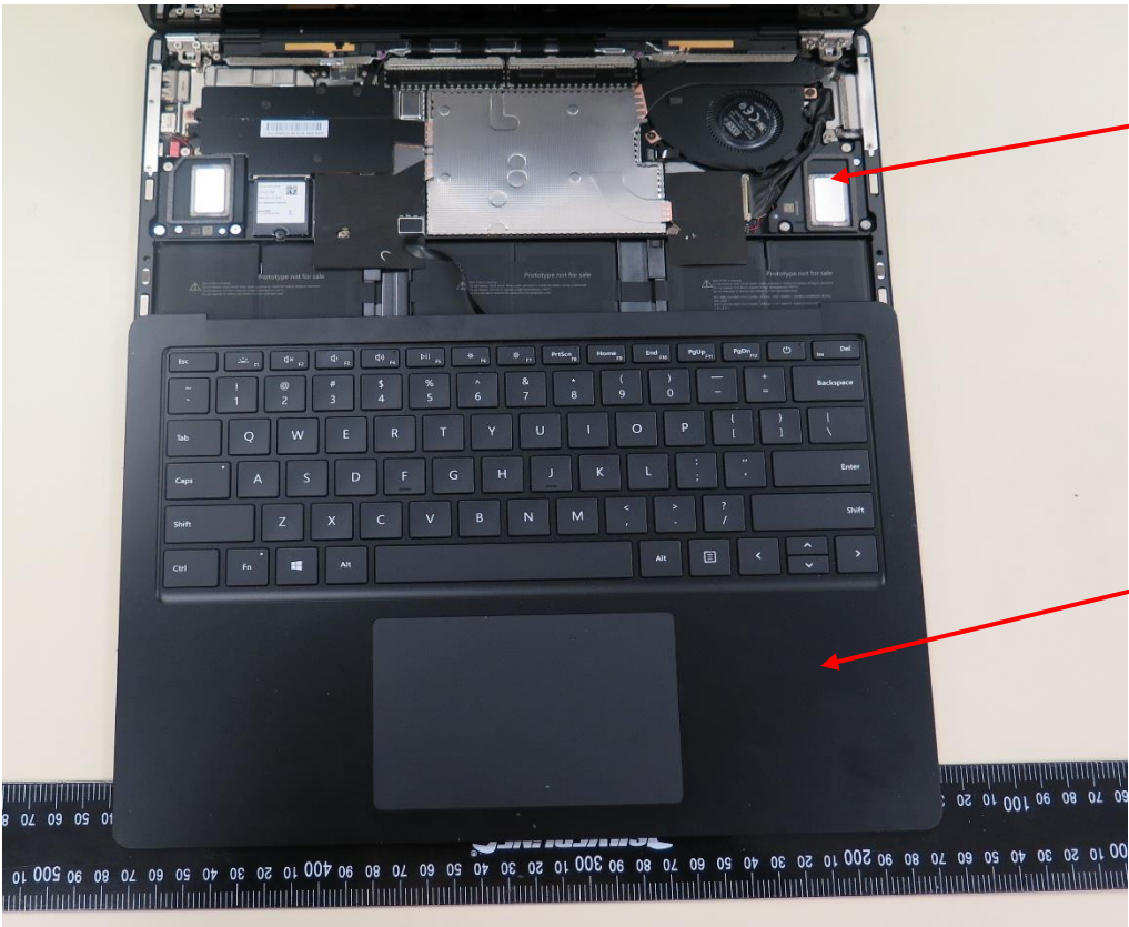
Figure 1 EUT with external housing off- showing main logic board
