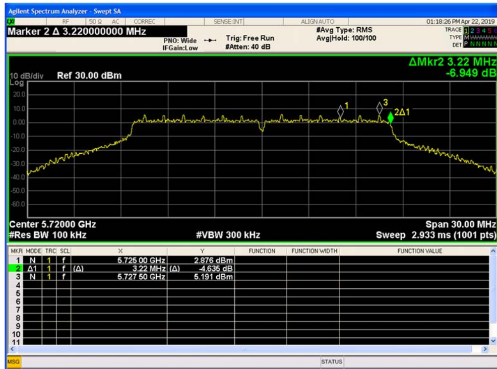
Figure 9-130 Bandwidth SISO Chain B 802.11a (Ch. 144)
