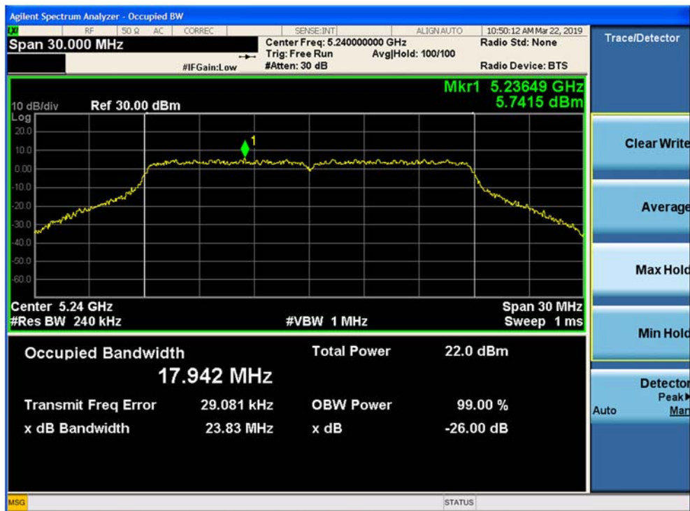
Figure 9-61. 26dB Emission Bandwidth and 99% OBW SISO Chain A 802.11ac VHT 20 (CH. 48)
