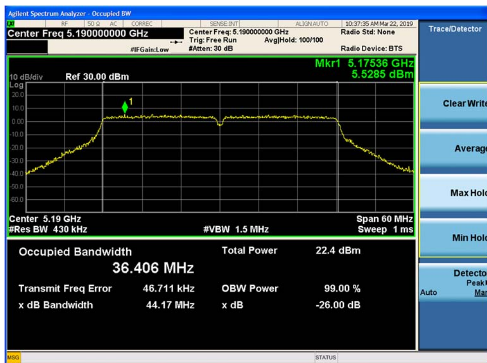
Figure 9-15. 26-dB Emission Bandwidth and 99% OBW SISO Chain A 802.11n HT40 (Ch. 38)
