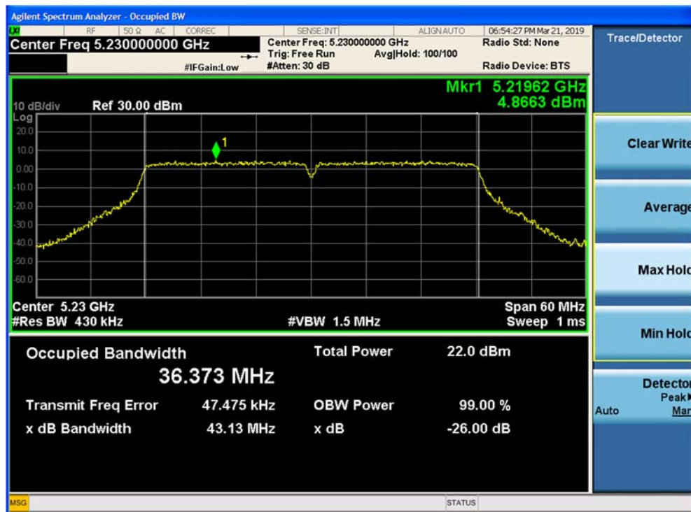
Figure 9-46. 26-dB Emission Bandwidth and 99% OBW SISO Chain B 802.11n HT40 (Ch. 46)
