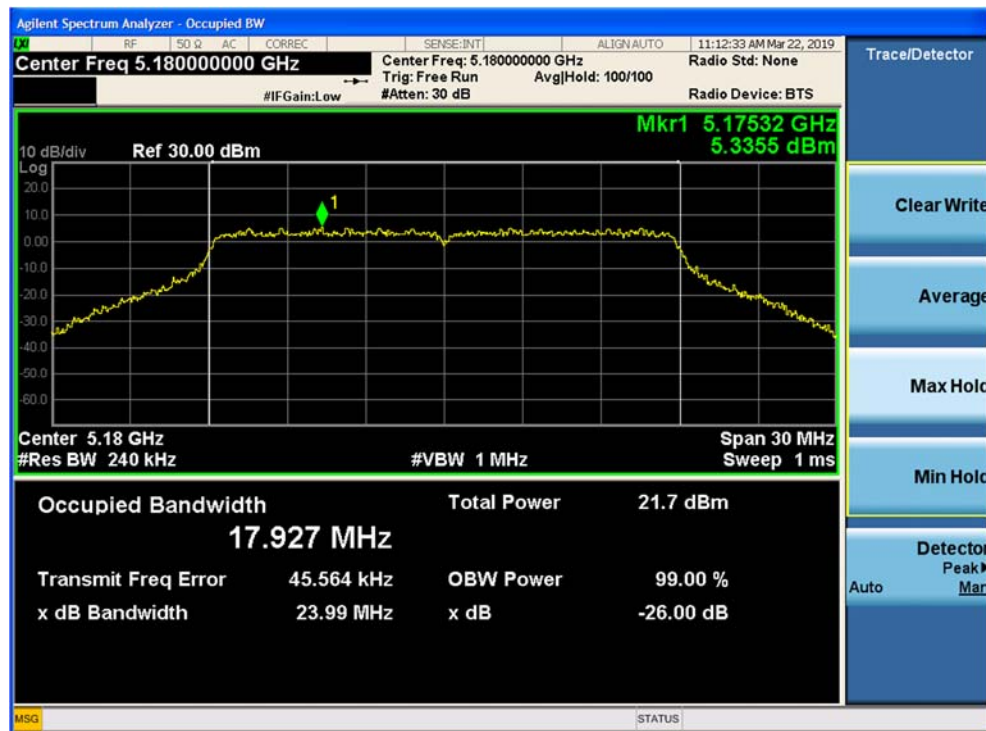
Figure 9-21. 26-dB Emission Bandwidth and 99% OBW SISO Chain A 802.11n HT20 (Ch. 36)
