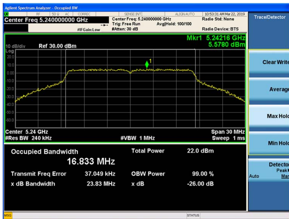
Figure 9-1 26-dB Emission Bandwidth and 99% OBW SISO Chain A 802.11a (Ch. 48)
