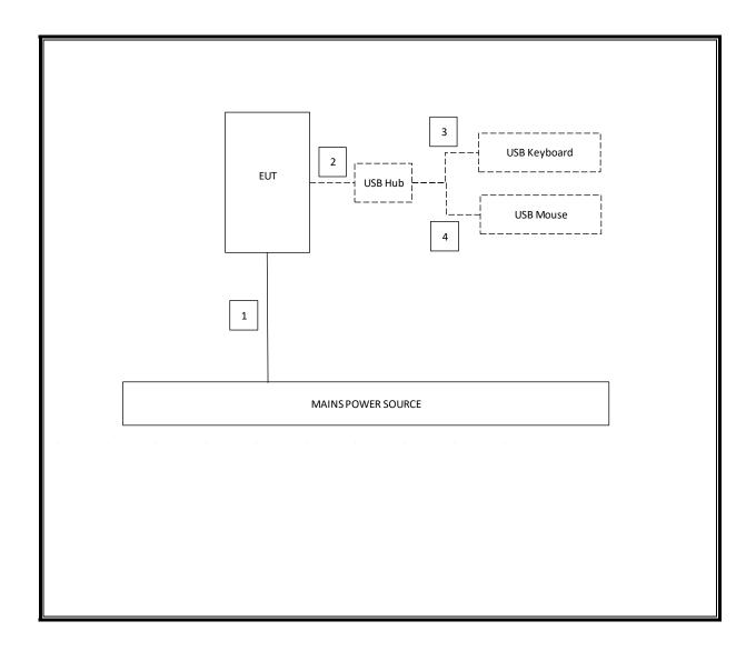
Lines and devices in dotted lines are not part of the EUT. Items used for placing EUT into test mode
