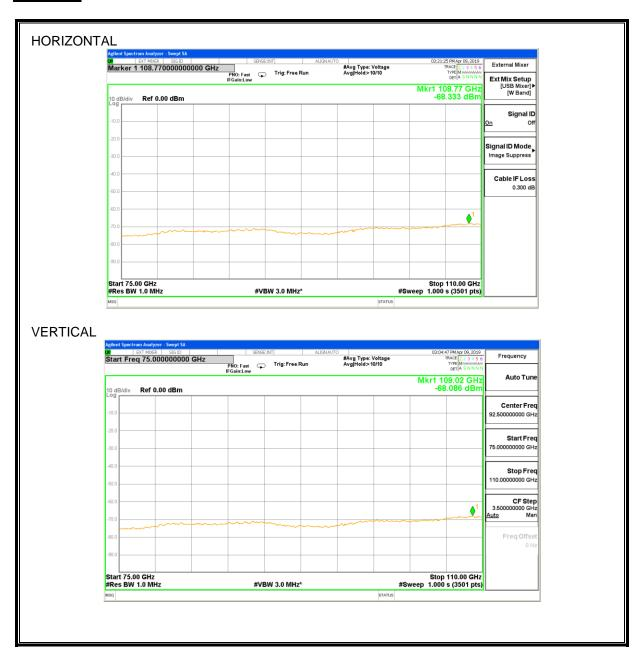
No emissions detected above the noise floor at 0.5 meters.
