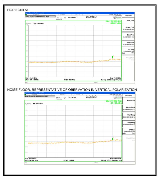
Except for third harmonic, no emissions detected above the noise floor at 1.0 meters.
