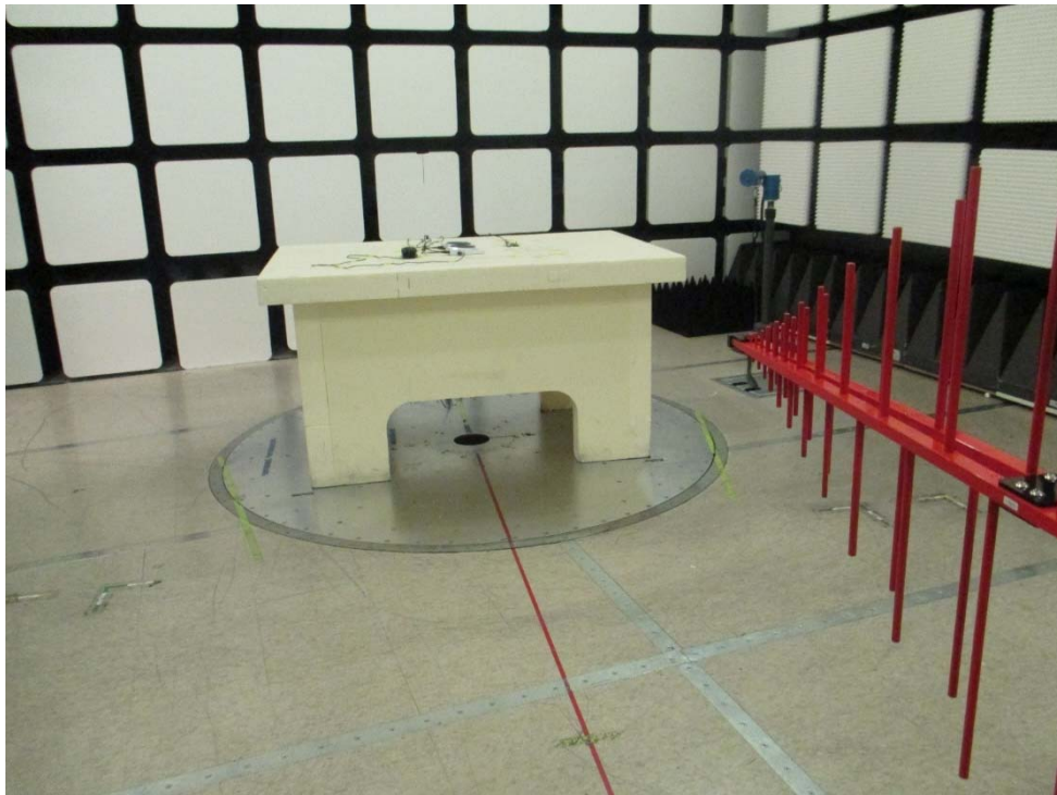
Fig.2 Radiated Spurious Emissions Test Setup (30MHz – 1GHz)
