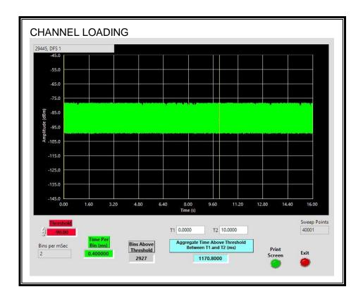
The level of traffic loading on the channel by the EUT is 11.70%
