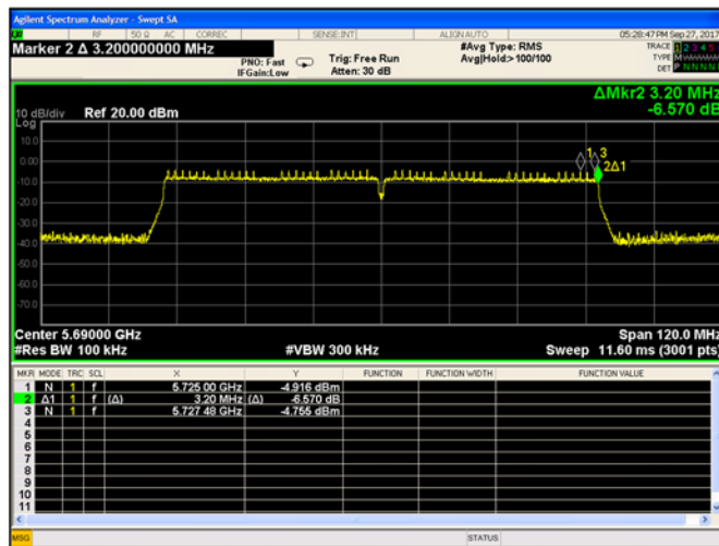
Plot 9-168. 6-dB Bandwidth Chain A 802.11ac VHT80 (Ch. 138)
