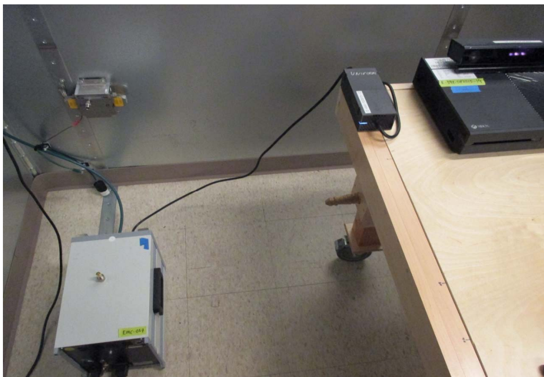
Fig. 10 AC Line Conducted Emissions Test Setup
