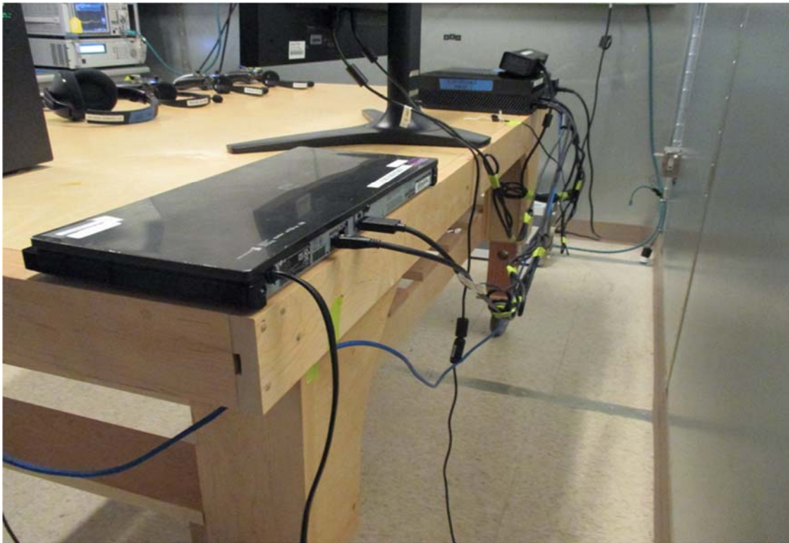
Fig. 11 AC Line Conducted Emissions Measurements Test Setup – Back View
