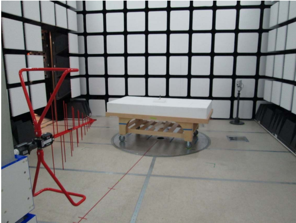
Fig.3 Radiated Spurious Emissions Test Setup (30MHz – 1GHz)
