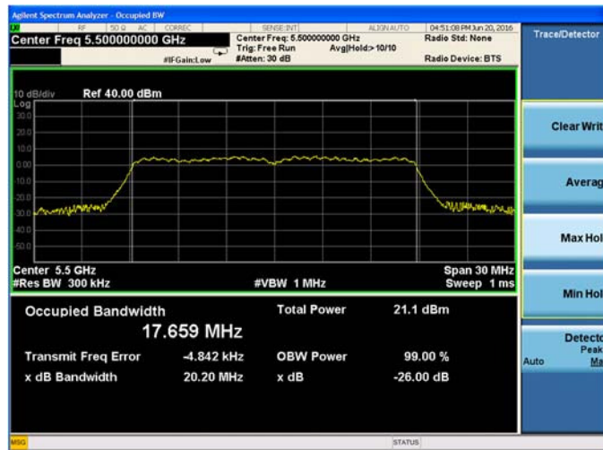
Plot 9-43. 26-dB Emission Bandwidth and 99% OBW Chain B 802.11n HT20 (Ch. 100)
