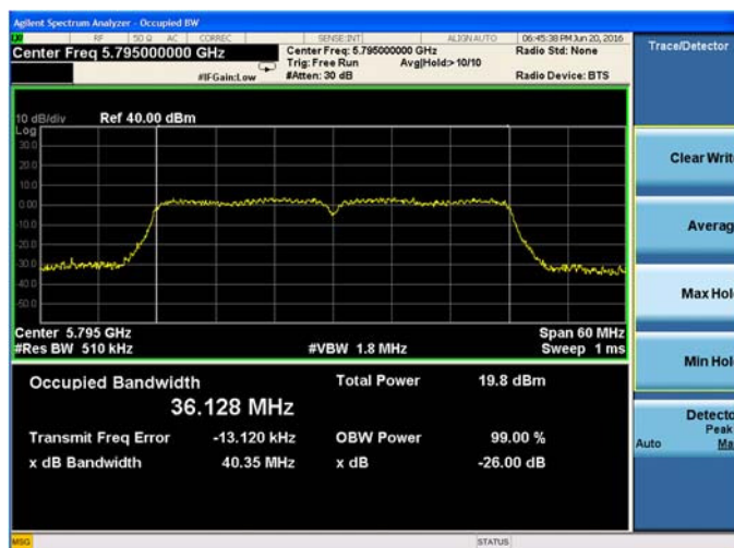
Plot 9-66. 26-dB Emission Bandwidth and 99% OBW Chain B 802.11n HT40 (Ch. 159)
