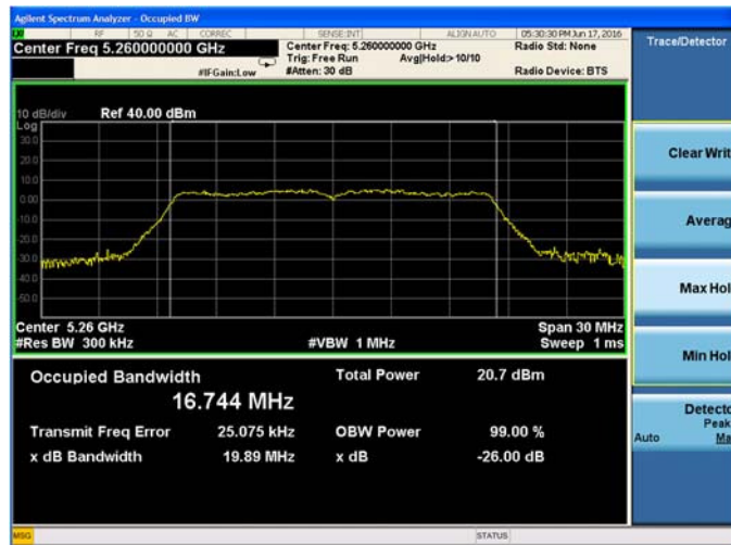
Plot 9-4. 26-dB Emission Bandwidth and 99% OBW Chain A 802.11a (Ch. 52)
