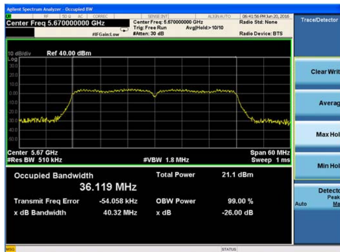
Plot 9-64. 26-dB Emission Bandwidth and 99% OBW Chain B 802.11n HT40 (Ch. 134)
