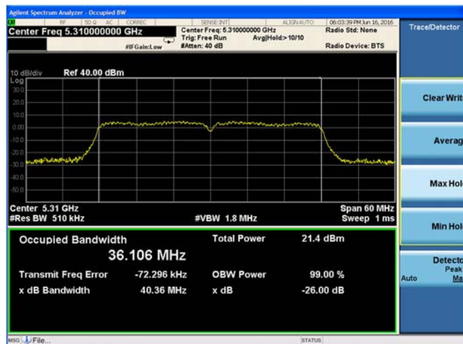
Plot 9-61. 26-dB Emission Bandwidth and 99% OBW Chain B 802.11n HT40 (Ch. 62)
