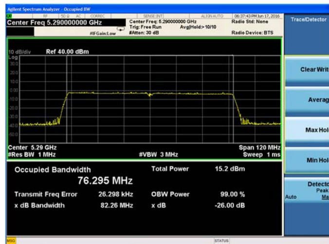
Plot 9-68. 26-dB Emission Bandwidth and 99% OBW Chain A 802.11ac VHT80 (Ch. 58)
