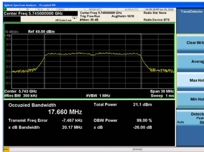
Plot 9-46. 26-dB Emission Bandwidth and 99% OBW Chain B 802.11n HT20 (Ch. 149)
