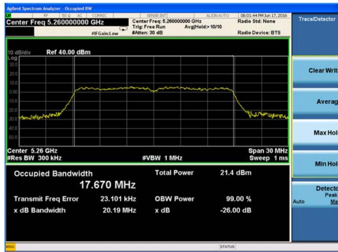
Plot 9-40. 26-dB Emission Bandwidth and 99% OBW Chain B 802.11n HT20 (Ch. 52)
