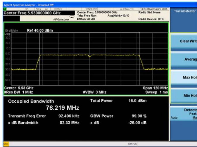
Plot 9-69. 26-dB Emission Bandwidth and 99% OBW Chain A 802.11ac VHT80 (Ch. 106)
