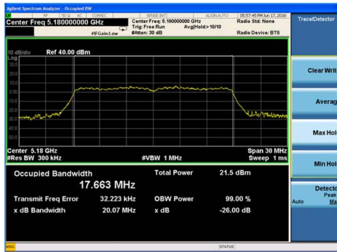
Plot 9-37. 26-dB Emission Bandwidth and 99% OBW Chain B 802.11n HT20 (Ch. 36)
