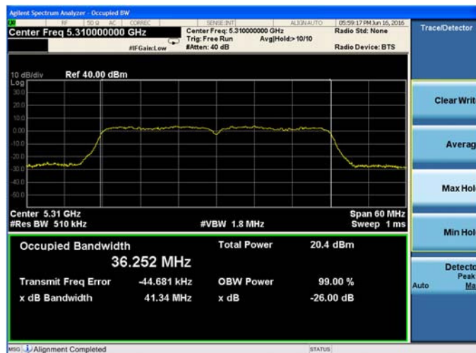
Plot 9-52. 26-dB Emission Bandwidth and 99% OBW Chain A 802.11n HT40 (Ch. 62)
