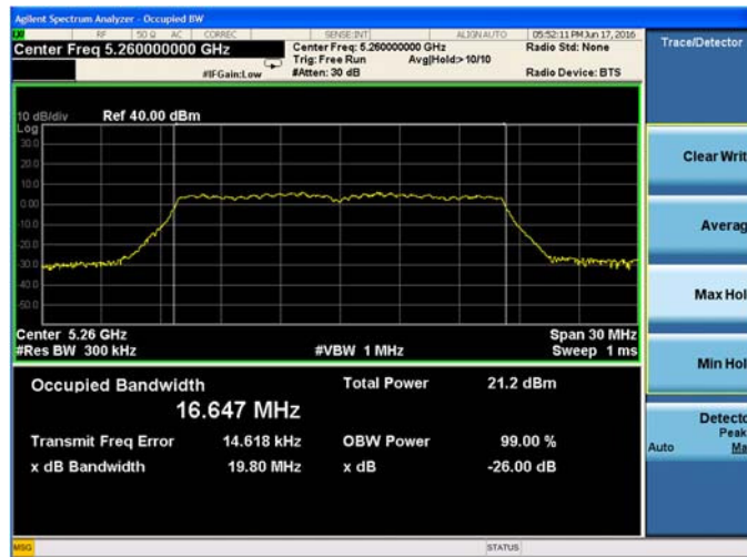
Plot 9-16. 26-dB Emission Bandwidth and 99% OBW Chain B 802.11a (Ch. 52)
