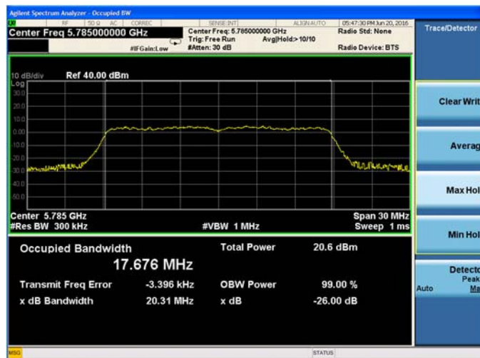
Plot 9-35. 26-dB Emission Bandwidth and 99% OBW Chain A 802.11n HT20 (Ch. 157)
