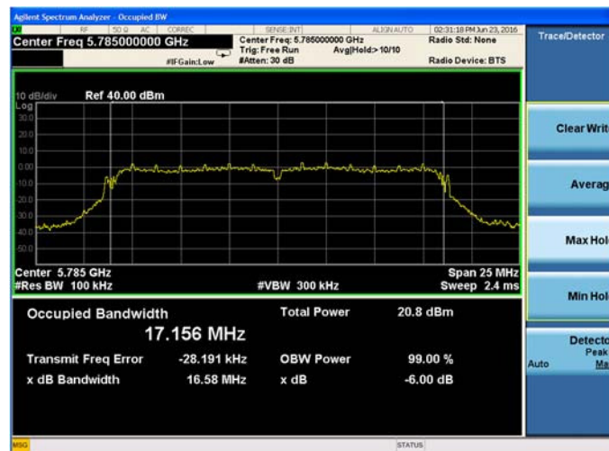
Plot 9-78. 6-dB Bandwidth Chain A 802.11a (Ch. 157)
