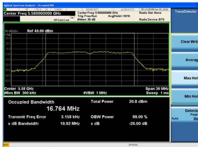
Plot 9-8. 26-dB Emission Bandwidth and 99% OBW Chain A 802.11a (Ch. 116)
