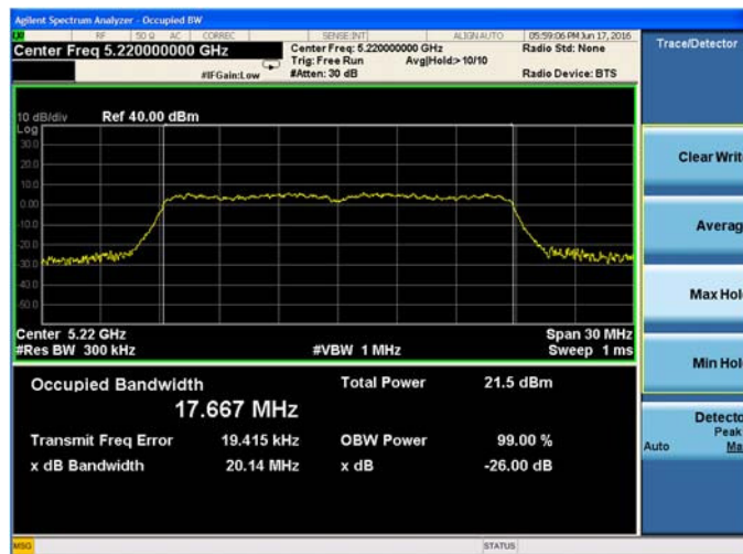
Plot 9-38. 26-dB Emission Bandwidth and 99% OBW Chain B 802.11n HT20 (Ch. 44)
