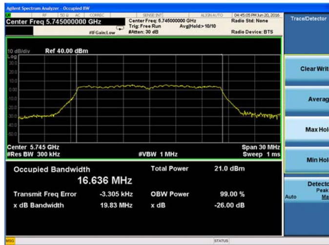
Plot 9-22. 26-dB Emission Bandwidth and 99% OBW Chain B 802.11a (Ch. 149)
