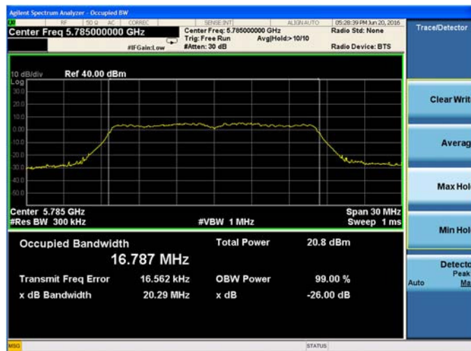
Plot 9-11. 26-dB Emission Bandwidth and 99% OBW Chain A 802.11a (Ch. 157)
