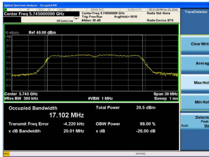
Plot 9-10. 26-dB Emission Bandwidth and 99% OBW Chain A 802.11a (Ch. 149)
