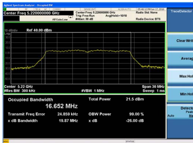
Plot 9-14. 26-dB Emission Bandwidth and 99% OBW Chain B 802.11a (Ch. 44)
