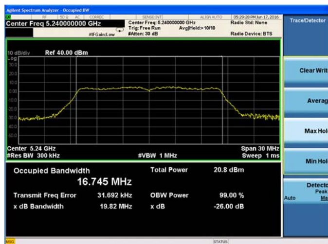
Plot 9-3 26-dB Emission Bandwidth and 99% OBW Chain A 802.11a (Ch. 48)
