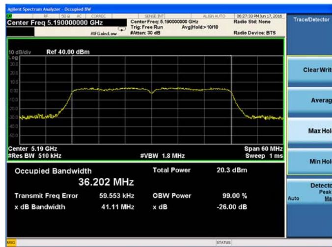
Plot 9-49. 26-dB Emission Bandwidth and 99% OBW Chain A 802.11n HT40 (Ch. 38)
