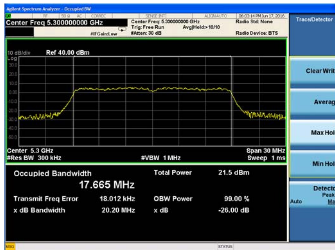
Plot 9-41. 26-dB Emission Bandwidth and 99% OBW Chain B 802.11n HT20 (Ch. 60)
