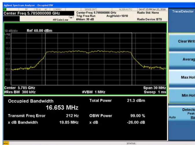
Plot 9-23. 26-dB Emission Bandwidth and 99% OBW Chain B 802.11a (Ch. 157)
