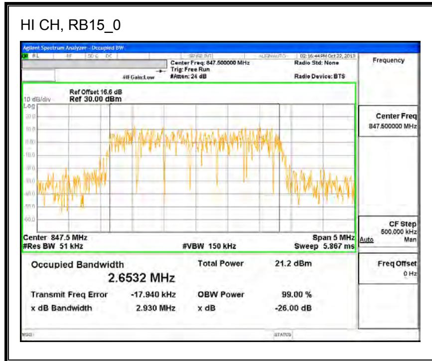
Band 5 (5MHz BANDWIDTH)LTE QPSK
