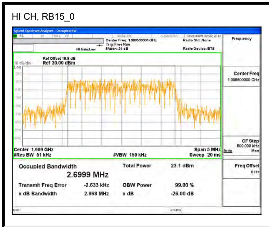
Band 2 (3MHz Bandwidth)LTE 16QAM
