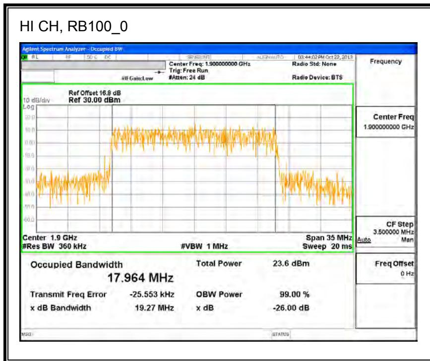
**Band 2 (20MHz Bandwidth)****LTE 16QAM**
