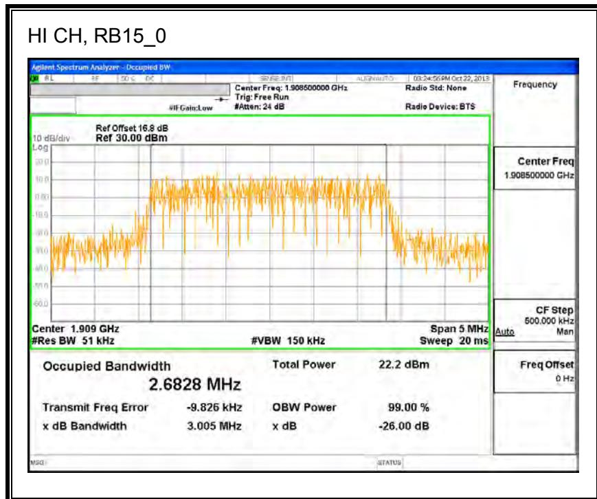
**Band 2 (5MHz Bandwidth)****LTE QPSK**
