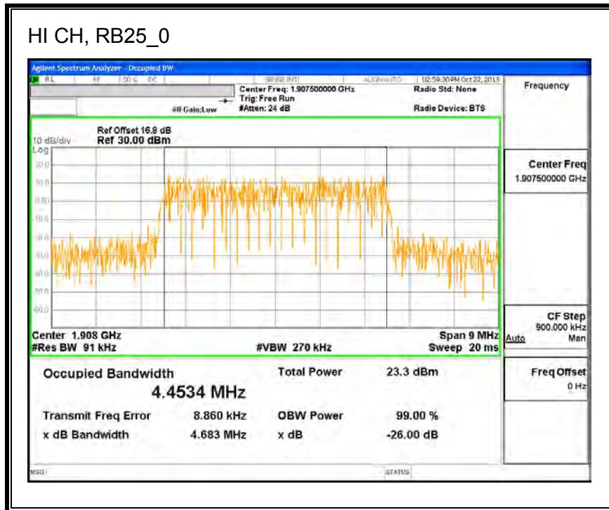
**Band 2 (5MHz Bandwidth)****LTE 16QAM**
