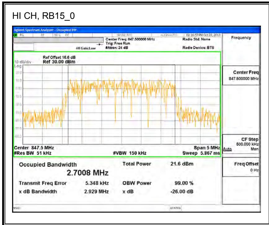
Band 5 (3MHz BANDWIDTH)LTE 16QAM
