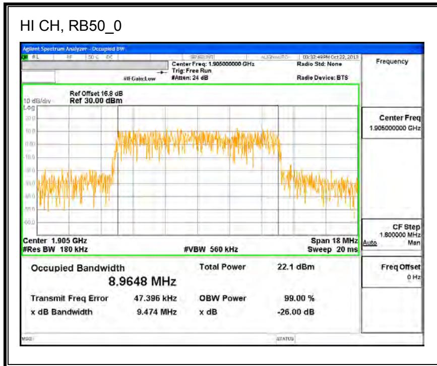
**Band 2 (15MHz Bandwidth)****LTE QPSK**
