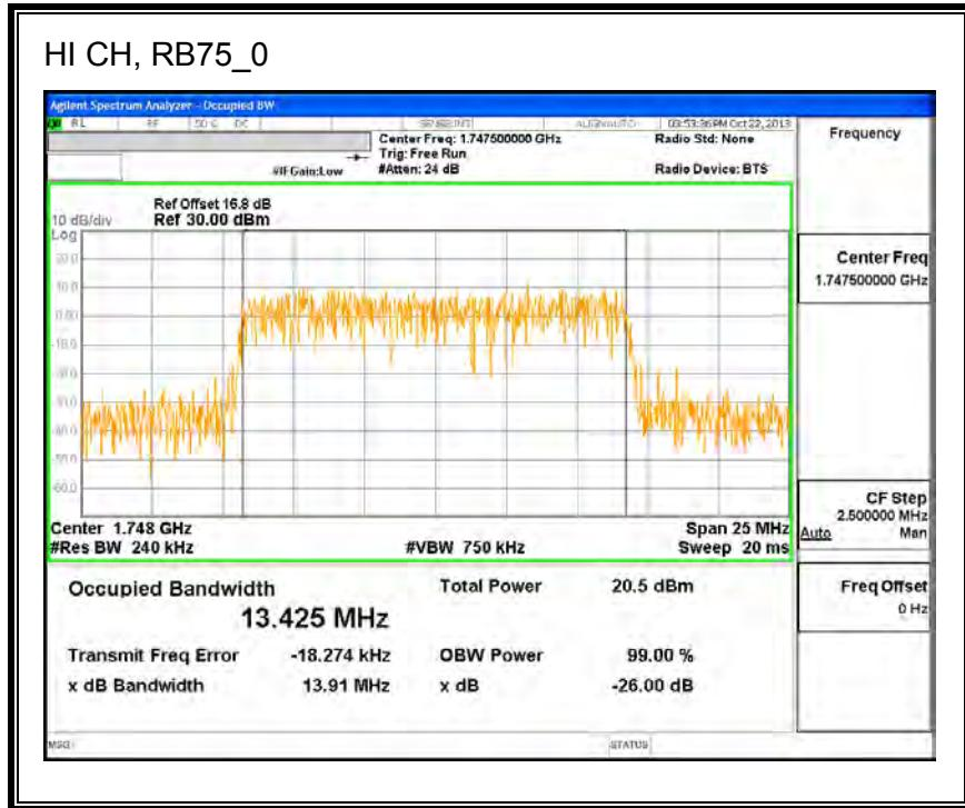
**Band 4 (20MHz Bandwidth)****LTE QPSK**
