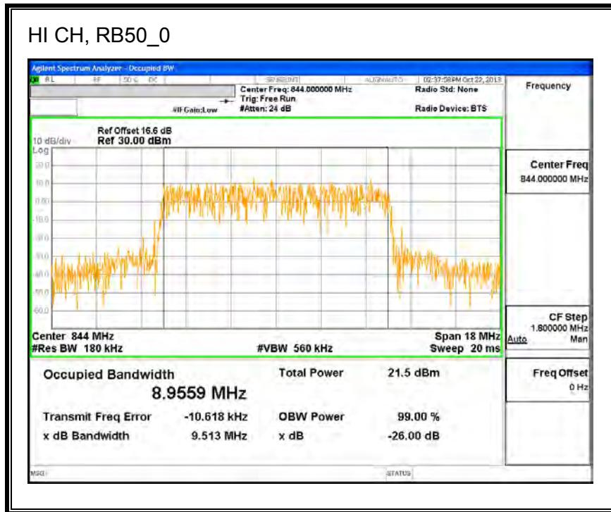
**Band 5 (10MHz BANDWIDTH)****LTE 16QAM**
