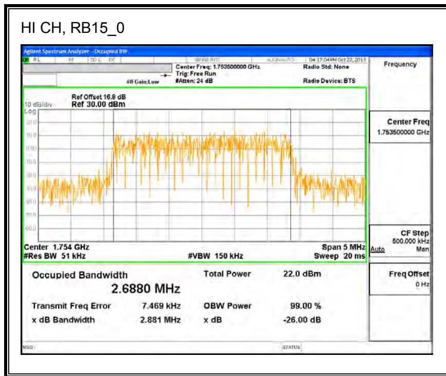
**Band 4 (3MHz Bandwidth)****LTE 16QAM**
