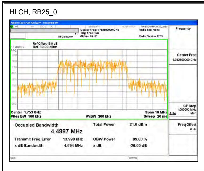
**Band 4 (5MHz Bandwidth)****LTE 16QAM**
