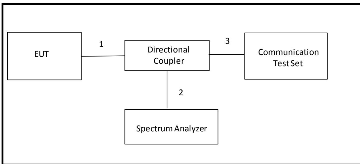
**RADIATED SETUP DIAGRAM FOR TESTS**
