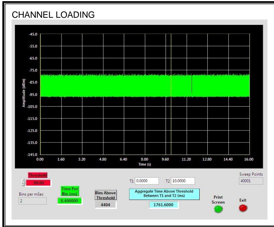
The level of traffic loading on the channel by the EUT is 17.61%
