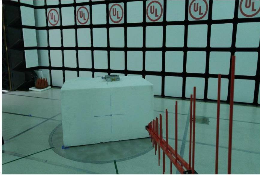
**RADIATED RF MEASUREMENT SETUP (ABOVE 1 GHz)**
