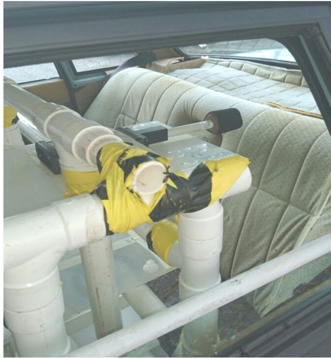
Test measurement setup for Passenger Back
