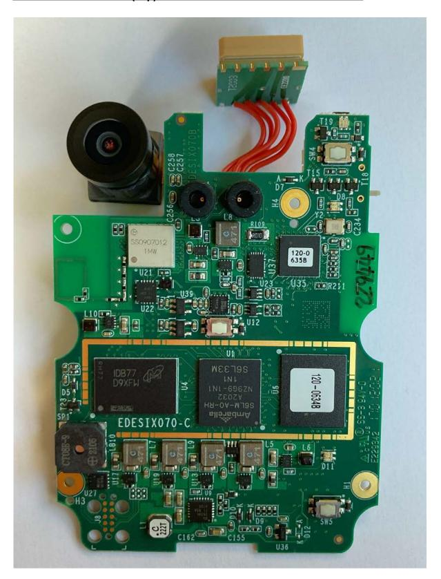
Exhibit 9D - Main PCB (Bottom) with GPS and Sensor Module attached
