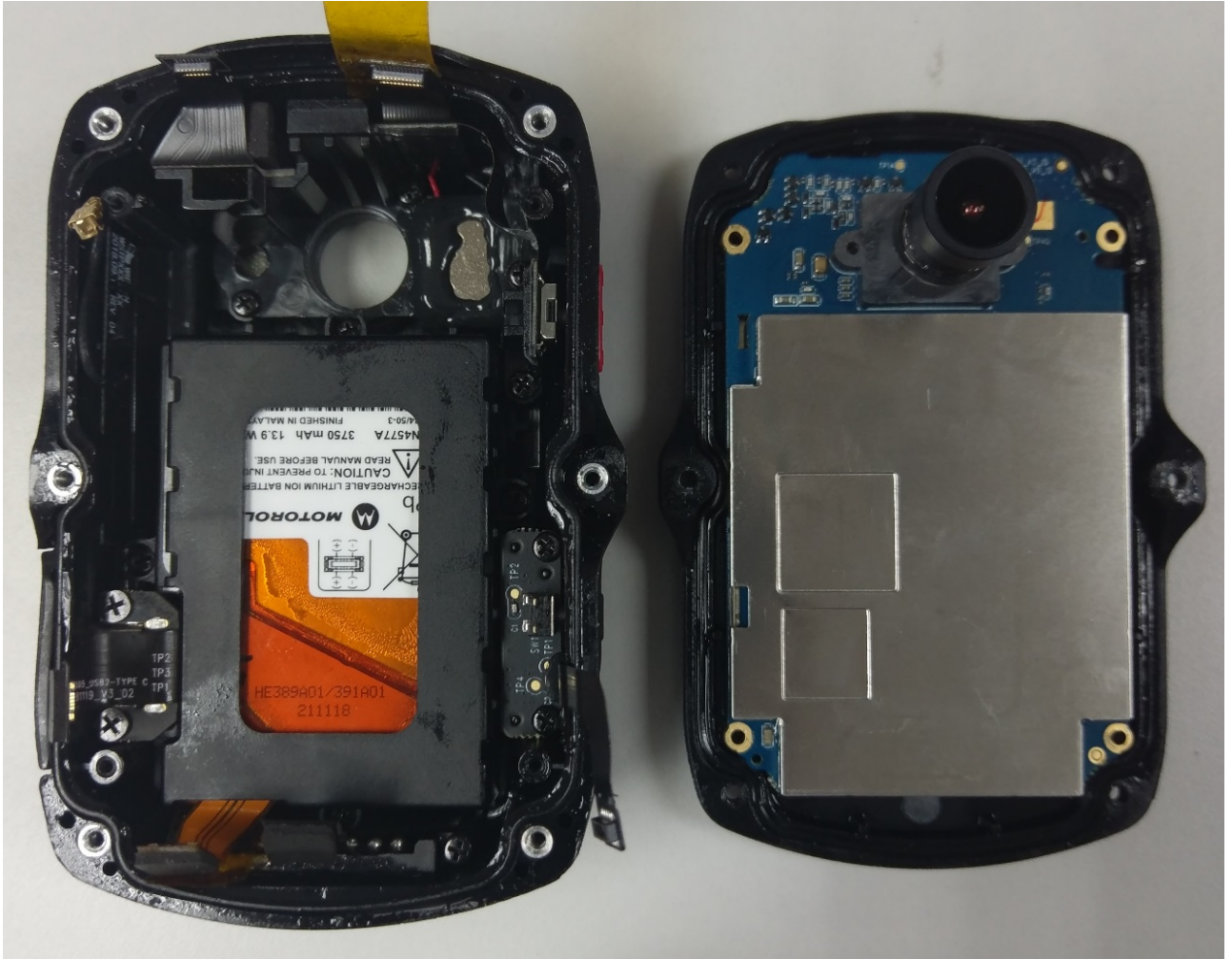
Exhibit 9F: Main board Front with Chassis with Battery in front housing
