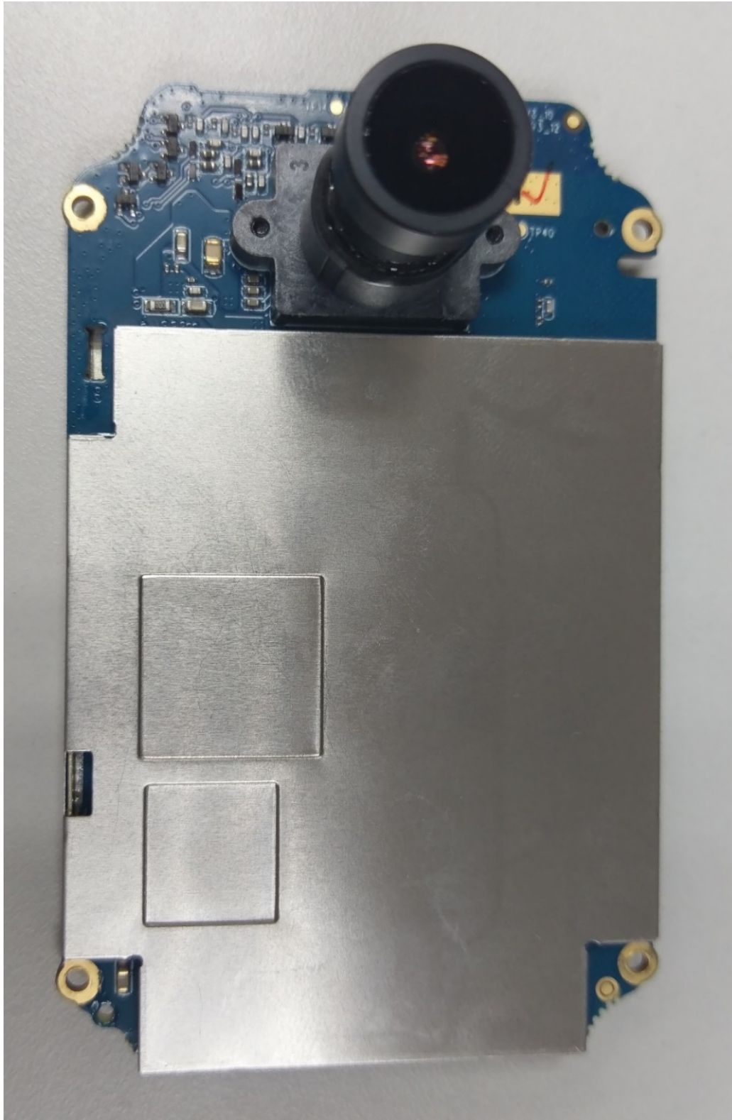
Exhibit 9A: Main board Front with Shields and Lens
