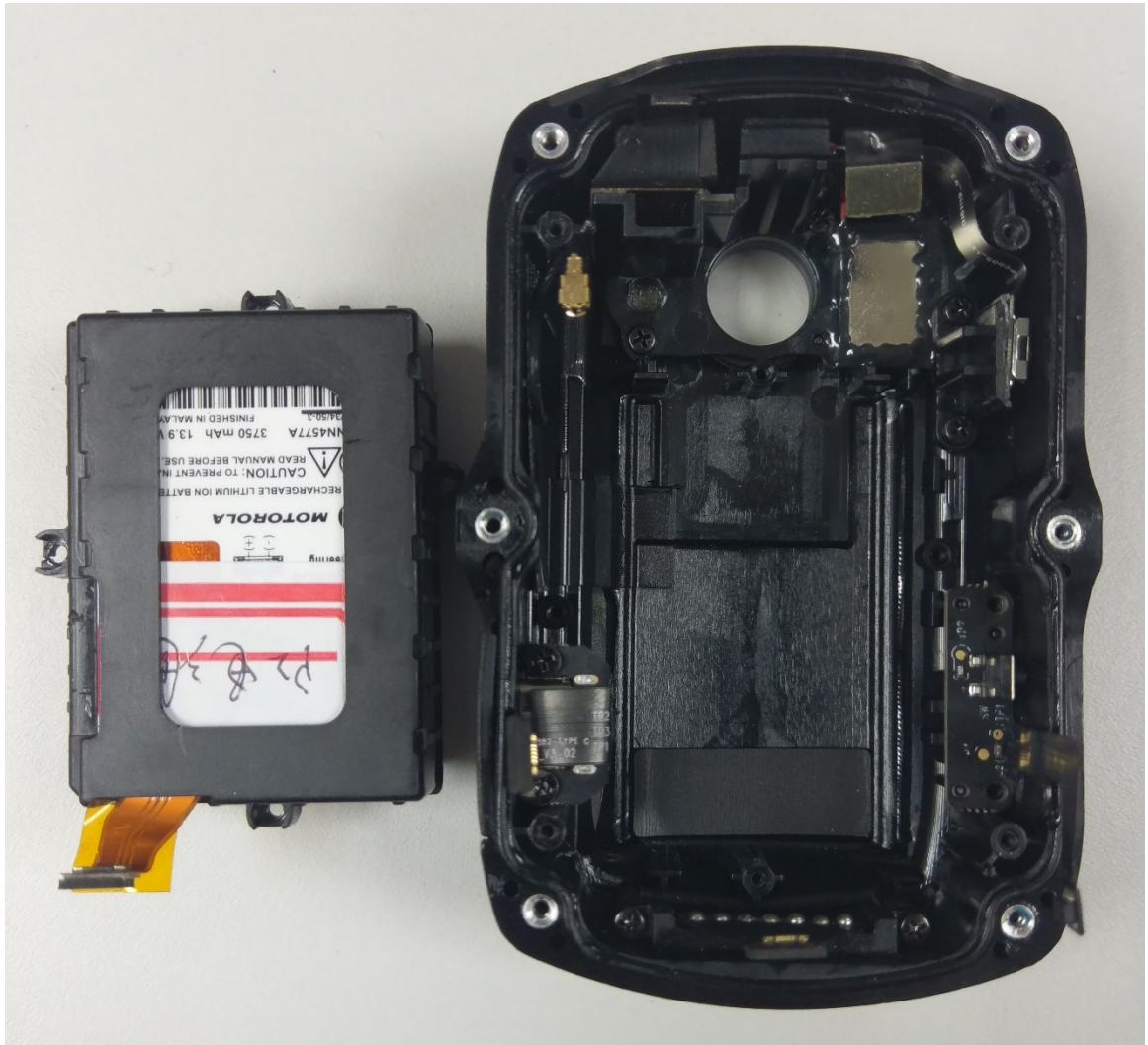
Exhibit 9G: Battery Pack and front housing without Battery Pack
