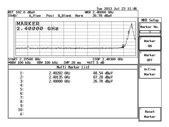
According to the page 13 of this report, the emission of the fundamental frequency 2402.0MHz is 89.3dBuV/m and 88.0dBuV/m for peak and average level respectively. Based on the delta method, the emission at the bandedge, 2400MHz, is more than 50dB below the fundamental and 20dB bandwidth falls in assigned band. It is deemed to comply with section 15.215. Besides, it is below the limit of 74dBuV/m and 54dBuV/m for peak and average level under 15.209. It is deemed to comply with section 15.249(d).
