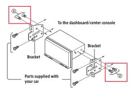
When mounting this unit to the preinstalled brackets of your car, use the mounting screws (2) in the appropriate screw holes based on your car: T for TOYOTA and N for NISSAN.
