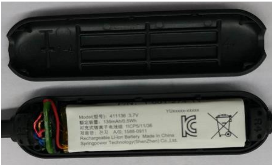
ASSY Box Battery Internal View
