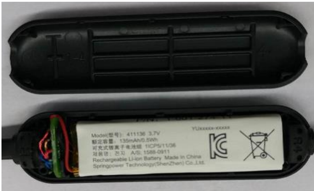
ASSY Box Battery Internal View
